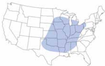
The shaded region on the map is the area affected by the 2015 IBC requirement for ICC 500 tornado shelters. Image courtesy of Huckabee
